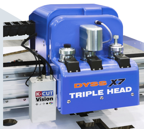
Triple head can house three tools simultaneously.
